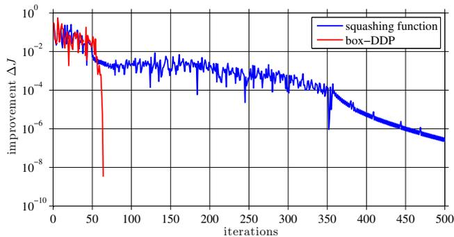
Fig. 4. Cost decrease  $\Delta J$  of the two algorithms for the car-parking problem. Box-DDP converges quadratically after 64 iterations, while the squashing-function solution has barely converged by 500.
