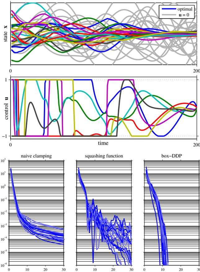
Fig. 2. Control-bounded random linear systems. Here  $h = 0.01$ ,  $n = 20$ ,  $m = 7$  and  $N = 200$ . **Top:** A typical state trajectory  $\mathbf{X} \equiv \{\mathbf{x}_0 \dots \mathbf{x}_{200}\}$ , the passive dynamics ( $\mathbf{U} = \mathbf{0}$ ) are shown in gray. **Middle:** the control trajectory  $\mathbf{U} \equiv \{\mathbf{u}_0 \dots \mathbf{u}_{199}\}$ . The limits  $\underline{\mathbf{b}} = -1$ ,  $\bar{\mathbf{b}} = 1$  are indicated.
